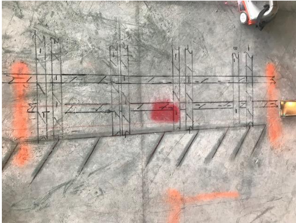
Scan #32/Denoted as 008: This scan shows an 8" slab with top and bottom layers of rebar.
