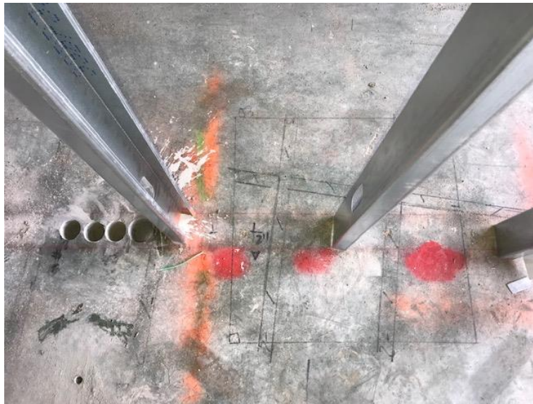
Scan #2/ Denoted as 03: This scan shows an 8" slab with a bottom layer of rebar.
