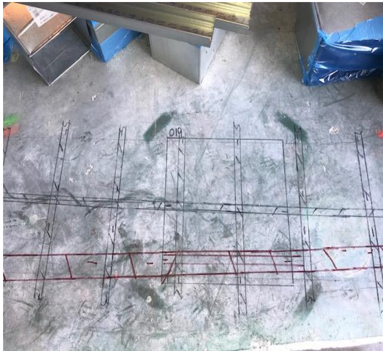
Scan #19/Denoted as 019: This scan shows an 8" slab with a top and bottom layer of rebar, and a possible conduit running horizontally through the grid.
