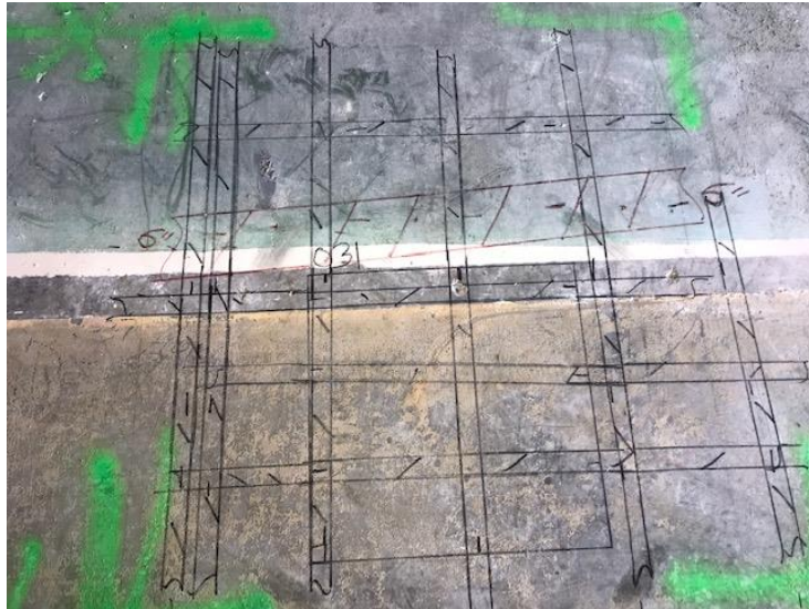
Scan #24/Denoted as 031: This scan shows a 9" slab with top and bottom layers of rebar, a possible conduit or cable, at a depth of 6" running horizontally through the slab.
