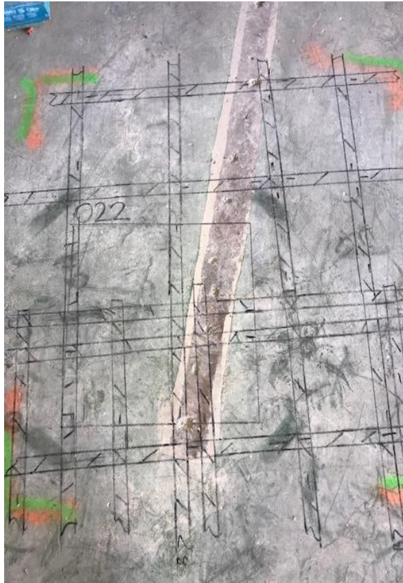
Scan #28/Denoted as 022: This scan shows an 8" slab with top and bottom layers of rebar.
