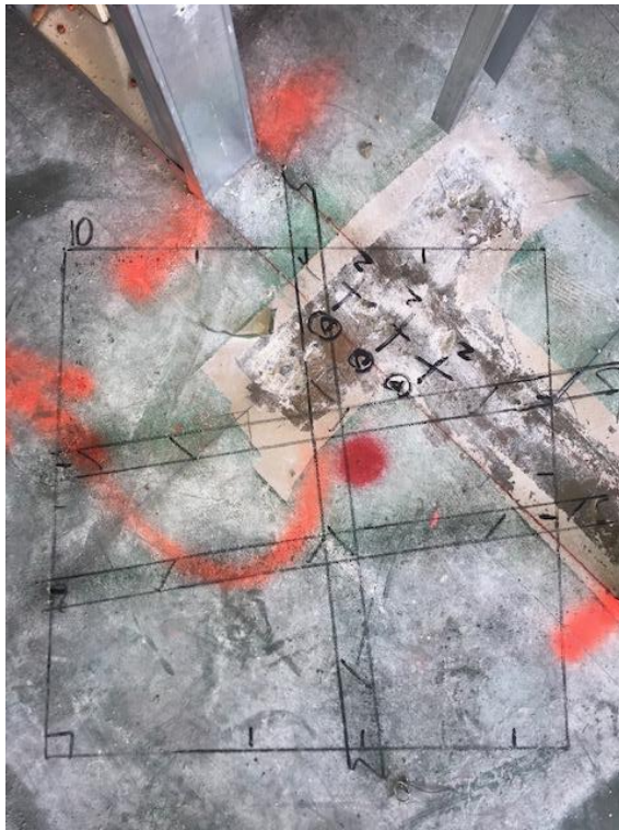
Scan #38/Denoted as 10: This scan shows an 8" slab with a bottom layer of rebar.
