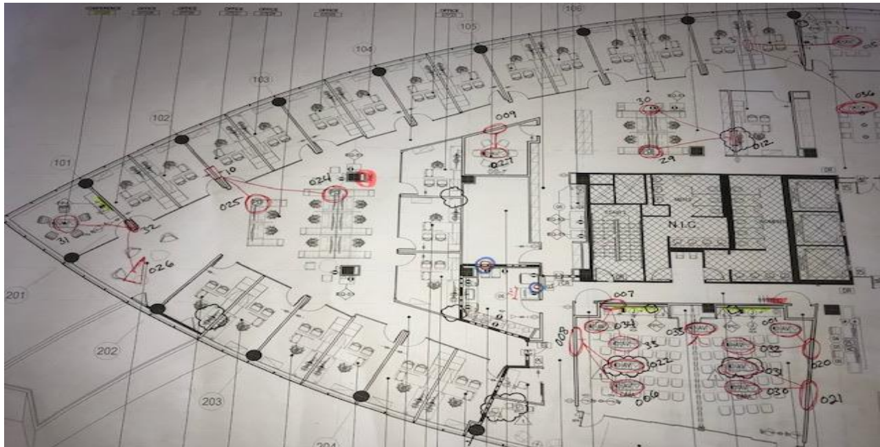
Image #1: This photo contains the south side of the existing 7 th floor plan, with approximately half of the 46 corresponding proposed penetration areas, marked in red, that were scanned using GPR.
